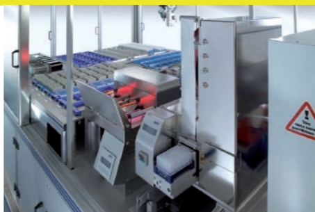
Dosage and Solution Preparation Station with tube sealing and capping.
